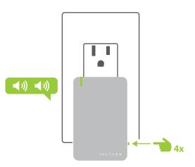
Inspect the status LED of a second Range Extender or any Dual-Band INSTEON device.
