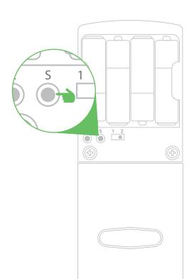
Tap the set button on Lock Controller. Your door lock will double-beep and the Lock Controller status LED will turn red.
