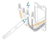
Turn off power and connect the corresponding wires from the junction box with the Insteon Wall Switch and cap them with wire nuts.
