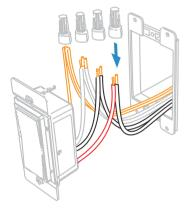
Install the Insteon Wall Switch. (5) attach the wall plate and turn on power.
