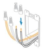
Turn on power and use a voltage detector to identify the live wire; this is your line wire.
