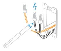
Turn off power and connect the corresponding wires from the junction box with the Insteon Wall Switch and cap them with wire nuts.
