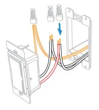
5 Install the Insteon Wall Switch, attach the wall plate and turn on power.
