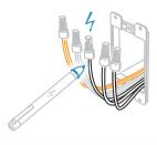
Turn off power and connect the corresponding wires. Refer to the reverse side for sense wire wiring.
