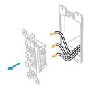
2 Unfold all of the wires from within the junction box. Separate the black wires and cap them with wire nuts.
