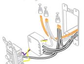
Reinstall your wall switch, attach the wall plate and turn on power.
