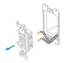
Unfold all of the wires from within the junction box.
