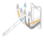
4 Turn off power and connect the corresponding wires. Refer to the reverse side for sense wire wiring.
