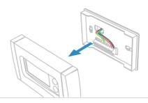
Take a picture of your thermostat's wires and apply the optional wire labels. Carefully remove the old mounting bracket.
