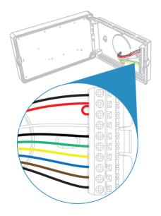
Wire colors may vary. Not all wires may be used. Match your wires to the labels printed on Insteon Thermostat.
