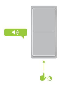
Make sure the device you wish to control is ON and then press and hold its set button until it double-beeps.
