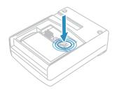
Motion Sensor's set button is inside the battery compartment.
