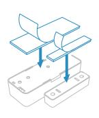
Position the sensor and magnet so that the arrows face and the gap is no more than ½ inch.
