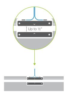
Route and secure the sensor wires along the opener rail back to the motor. Plug the I/O Linc and garage door motor into power.
