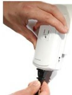
NOTE: After completing installation, you will not be able to use the load's built-in switch to control the load unless Load Sensing is enabled. See *Enabling/Disabling Load Sensing*.
